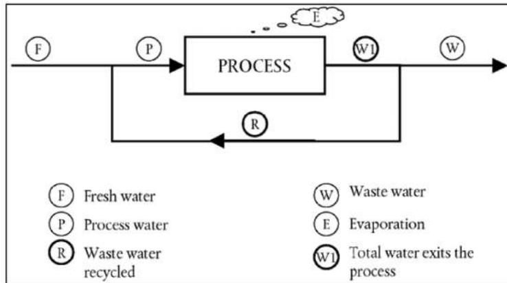
Figure A1: Water flow scheme that shall be used to calculate water recycling ratio <sup>(1)</sup>
